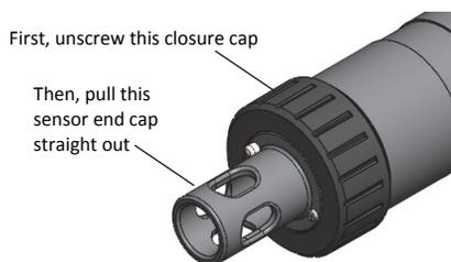
2. If this is the first time you’re installing a pH electrode, skip to step 3. If a pH electrode is currently installed, gently remove it from the sensor end cap. Use a foam swab dipped in water to clean the internal O-rings. Use the foam swab to spread a small dot of silicone-based grease along both the O-rings inside the sensor end cap. Do not use a cotton swab as the fibers on the swab can interfere with the operation of the electrode.
