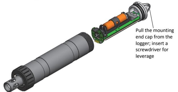
4. Remove the battery strap. Insert a flat-head screwdriver into the hole on the strap to lift it off the battery.
