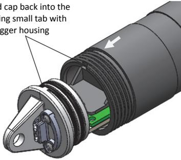
Mounting end cap installed with correct alignment
