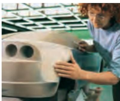
High-quality master models made of SikaBlock® M600 N / 700 N provides highest dimensional accuracy
