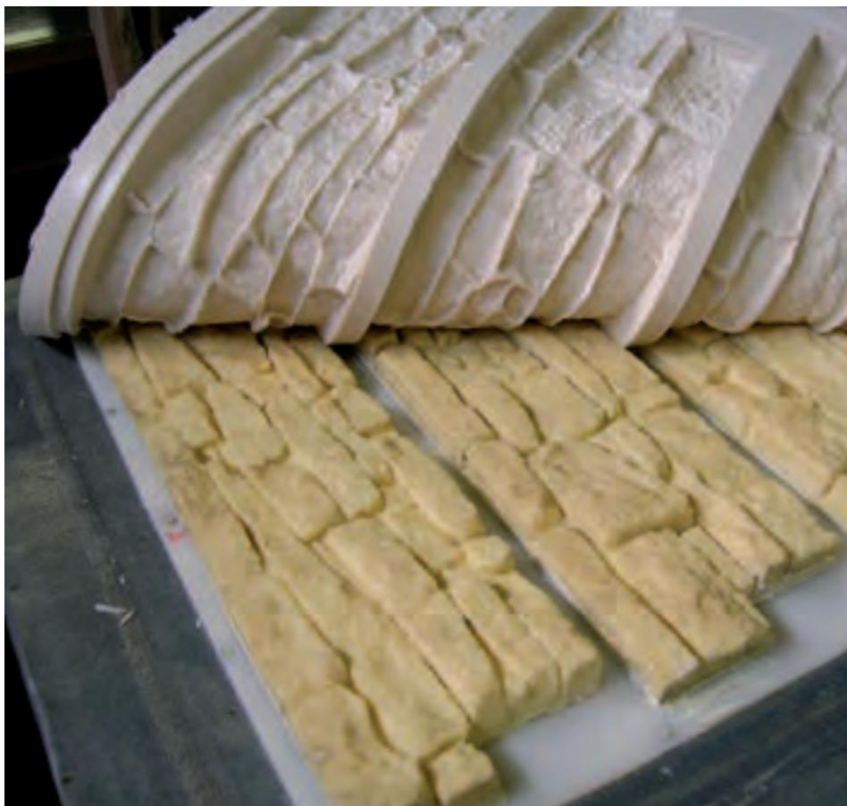
Release of SikaBiresin® UR548 soft mould for stone facing
