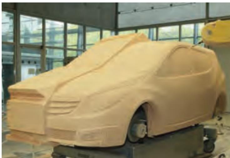
Full scale car model made of SikaBlock® M330 boards bonded with SikaBiresin® B260
