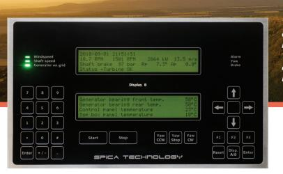
The Spica Retrofit Controller comes with a dual display. It has the same structure as a TAC controller which makes it easy to operate and turbine maintenance more effective.
