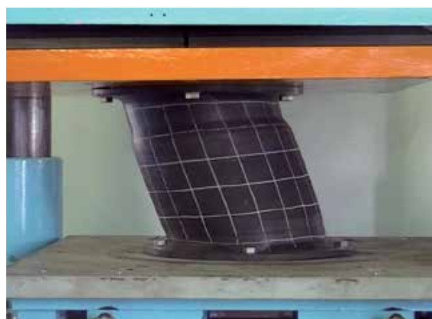
CSS Fender shear testing with panel and UHMW-PE face pads
