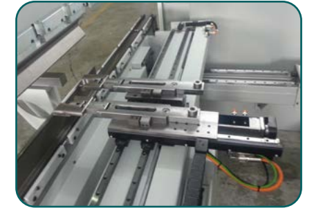
5-axis back gauge, X-X'-R-Z1-Z2 (optional)
