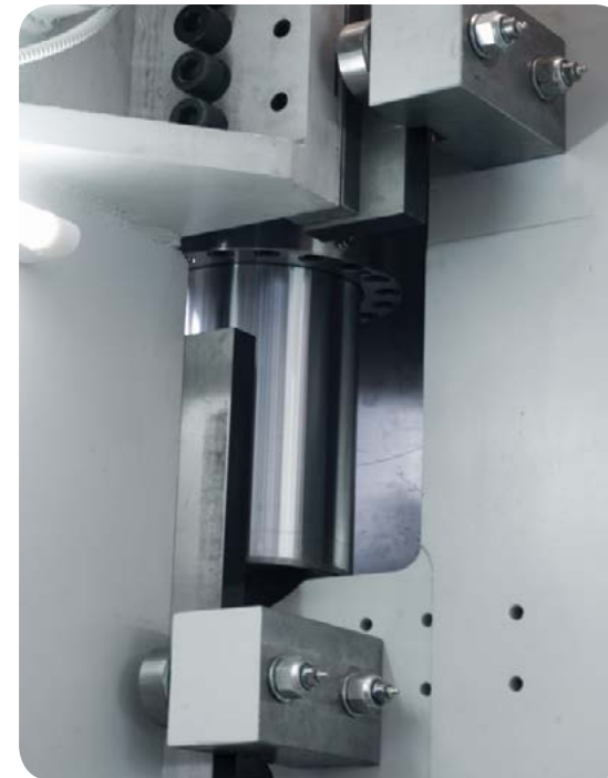
Double upper and lower roller bearing for accurate and fast beam movement.
