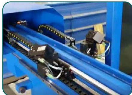
i-measure: Laser measurement of the bending angle and real time correction (optional)
