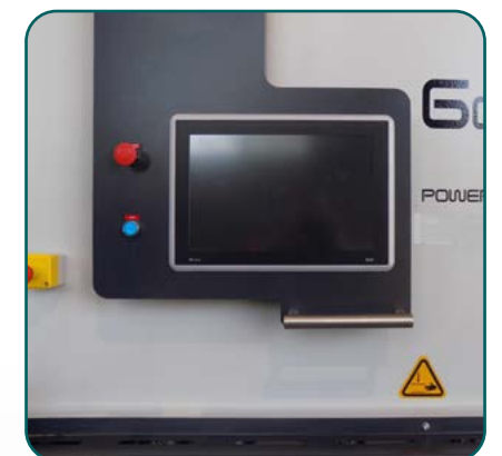
Color Touch Screen 15", movable along machine's length (optional)
