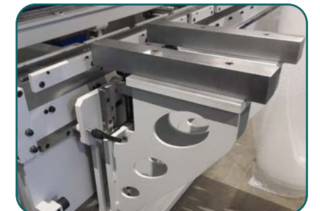
Heavy-duty front supports, moveable on linear guide, height adjustable (optional)
