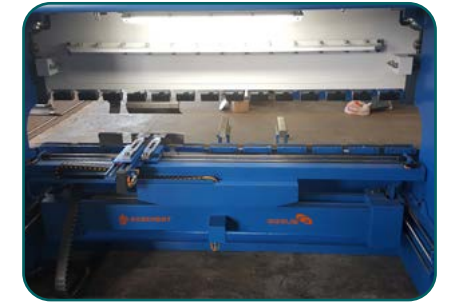
Back gauge guiding system on machine's sides (free space at the back)
