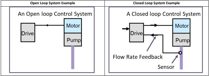
Optidrive E3 has a built-in flexible PI controller that can be used for a variety of process control applications. Typical applications include pressure control, flow rate control, temperature control etc. In addition, more complex functions, such as differential pressure, constant motor current or even maintaining the DC link voltage for simple solar pumping applications can be achieved. This document describes the setup procedure for each of the operating modes available.
