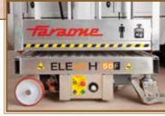
Without outriggers reaches the machine a working height of up to 3.8 m. This is automatically controlled, using sensors that detect the height of the basket.
