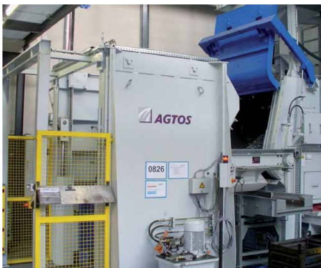
Steel mill tumble belt shot blast machine type MR 550 with loader and vibro chute for processing of engine components
