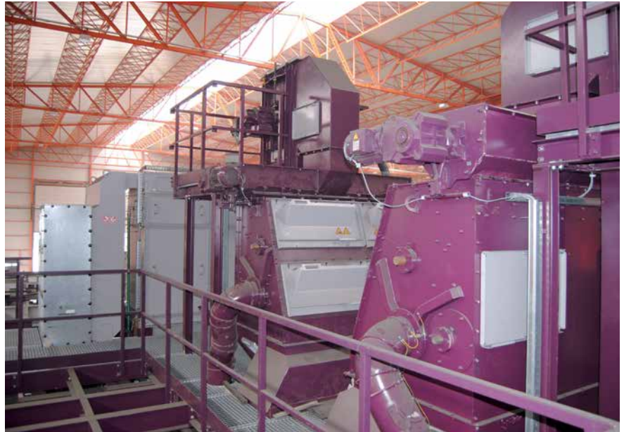
Fig. 2: Magnetic/air separation in a large foundry facility
