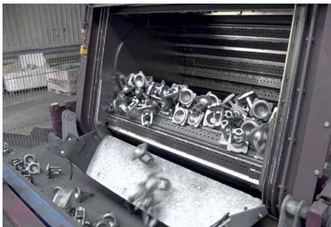
Steel mill tumble blast machine of type MR 0270 for cast workpieces
