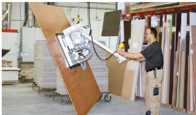
VacuMaster Multi for swiveling wooden boards by 90°
