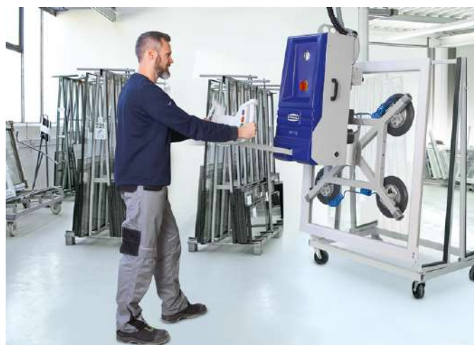
Vacuum lifting device VacuMaster Window Comfort for handling windows, glass panes and glass components up to max. 500 kg
