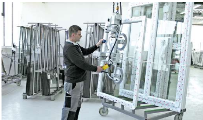
VacuMaster Window for rotating and palletizing windows
