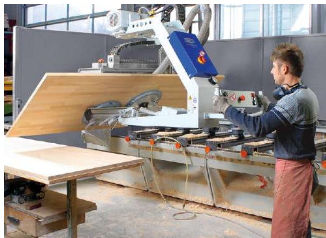
Vacuum lifting device VacuMaster Comfort for turning coated wooden boards by 180°
