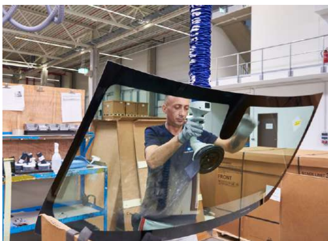
Vacuum tube lifter JumboFlex for handling windshields
