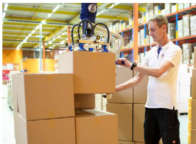
Vacuum tube lifter JumboFlex High-Stack for safe handling of various workpieces at stacking heights of up to 255 cm
