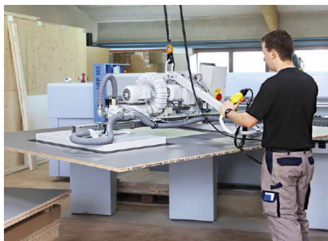
Vacuum lifting device VacuMaster Multi with 90° swivel angle for handling heavy, porous wooden boards
