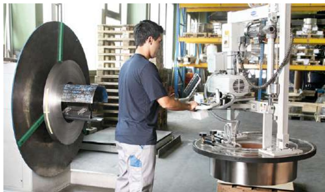
VacuMaster Coil for swiveling stainless steel coils by 90°
