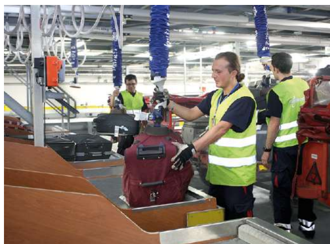
Airport | Vacuum tube lifter JumboFlex for handling of luggage pieces
