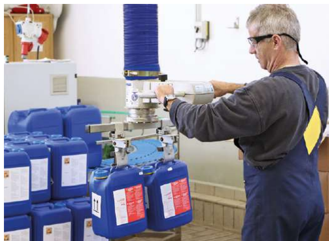
Vacuum tube lifter JumboErgo with mechanical gripper for handling jugs
