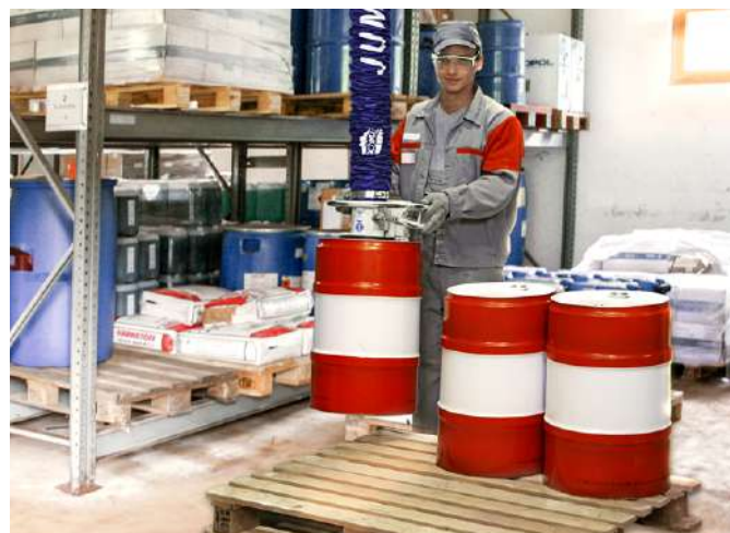
Vacuum tube lifter JumboSprint for handling barrels
