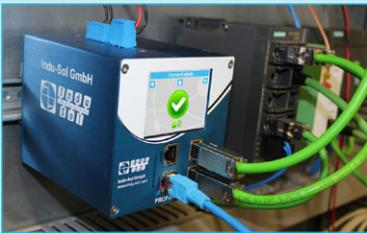
Fig. 1: Installation of the PROFINET-INspektor® NT
