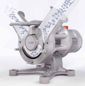
A single sinusoidal rotor creates four evenly sized chambers. As each chamber rotates it gently conveys the fluid from the inlet port to the outlet port. At the same time, the opposite chamber opens to draw in more fluid, resulting in a smooth flow with virtually no pulsation.
