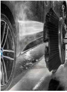
**High-pressure wheel sill wash device** Removes the majority of dirt
