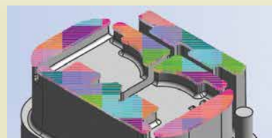
Scanning cell size, cell order, and direction can be customized.
