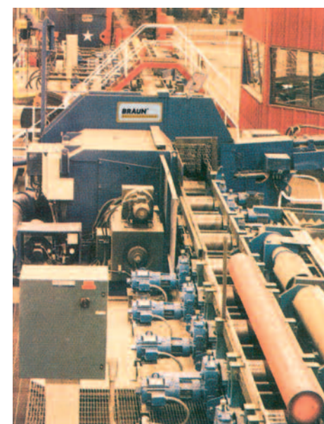
Fig. 32 Chop-stroke cut abrasive cut-off machine type TS 15 V with entry and exit end material handling equipment at SCOT FORGE, Spring Grove, IL, USA; cutting wheel diameter max. 1500 mm (59 in), material: forged bar, diameter 150 to 420 mm (6 to 16-1/2 in), cutting temperature max. 1000 °C (1832 °F).
