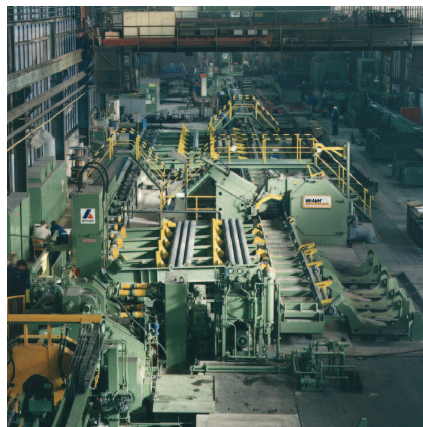
Fig. 27 Complete installation with chop-stroke abrasive cut-off machine type TS 15 V, in forging/conditioning area at BÖHLER Edelstahl, Kapfenberg, Austria
