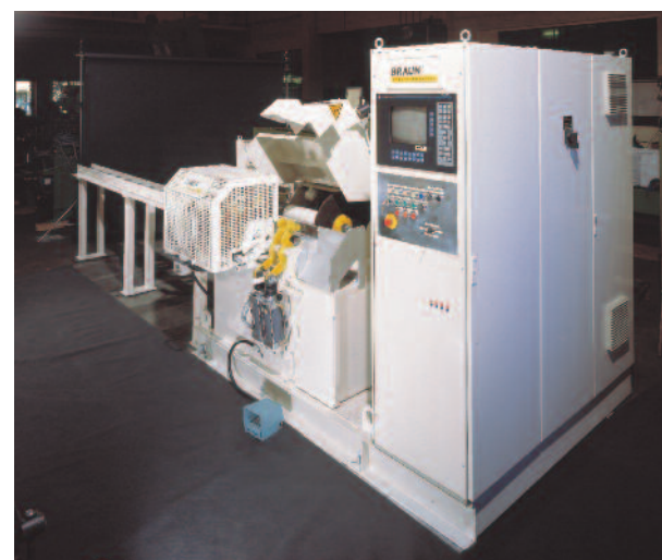
Fig. 37 Chop-stroke abrasive cut-off machine, type TS 5 V in compact form for test laboratory at NORTON Abrasives, USA; cutting wheel diameter max. 500 mm (20 in), material: bar stock, diameter max. 60 mm (2-3/8 in), cutting temperature max. 100°C (212 °F).
