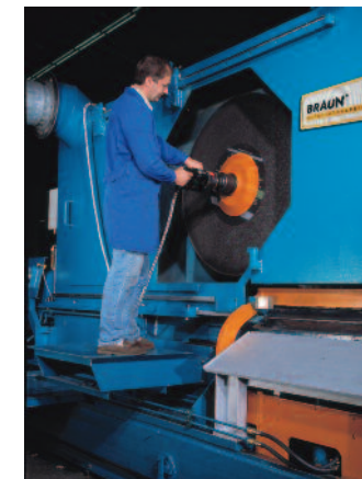
Fig. 21 Pneumatic wrench hammer for changing cutting wheels (option)
