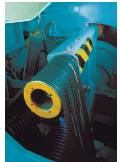
Fig. 20 Cutting shaft driven by multiple V-belts (up to machine size TS 8)
