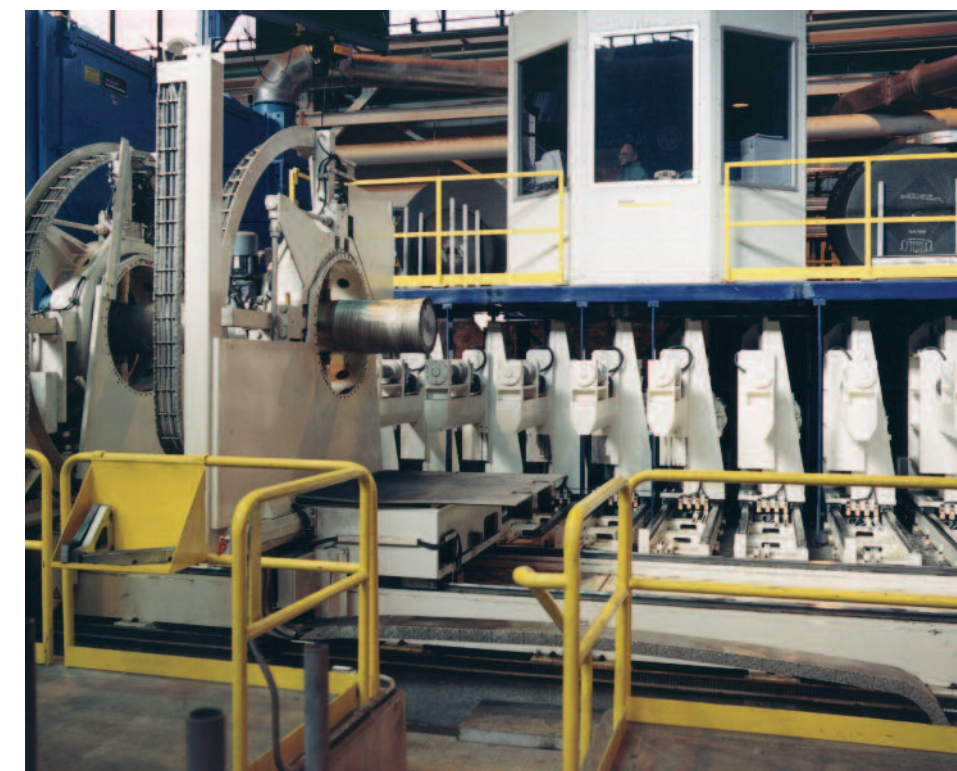
Fig. 28 Complete installation with 2 chop-stroke abrasive cut-off machines type TS 16 W, at CARPENTER Technologies, Reading, PA, USA; view of rotating chucks for inverting large ingots during index cutting
