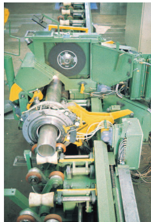
Fig. 36 Chop-stroke abrasive cut-off machine type TS 6 V with rotating chuck and specially-designed material feed and transfer system to rotary-cut tubes at SCHÖLLER-BLECKMANN, Ternitz, Austria; cutting wheel diameter max. 600 mm (24 in), material: stainless steel tube, diameter 60 to 280 mm (2-3/8 to 11 in), cutting temperature max. 100°C (212 °F).
