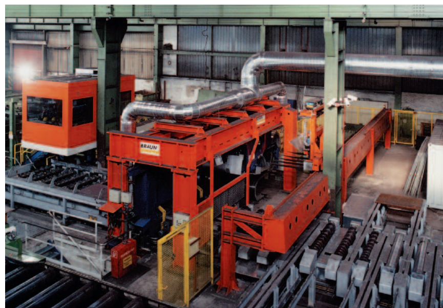
Fig. 31 Gantry-type traverse abrasive cut-off machine type TS 12 FP at BÖHLER Bleche, Mürtzschlag-Hönigsberg, Austria; cutting wheel diameter max. 1260 mm (49-1/2 in), plate width up to 2300 mm (90-1/2 in), material thickness max. 260 mm (10-1/4 in), cutting temperature between 600 and 1000°C (1112 and 1832 °F); slabs can also be cold-cut
