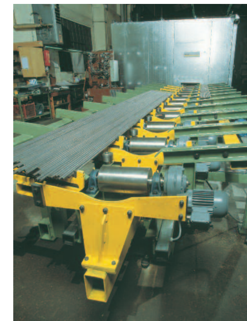
Fig. 33 Chop-stroke abrasive cut-off machine type TS 6 V with integral material handling system at DONETSKIJ METALURGICESKIJ ZAVOD, Donetsk, Ukraine; cutting wheel diameter max. 600 mm (24 in), material: bar, diameter 10 to 25 mm (0-3/8 to 1 in), cutting temperature max. 100 °C (212 °F).
