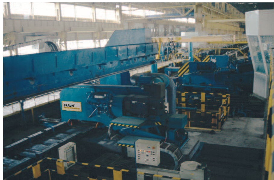
Fig. 30 Traverse abrasive cut-off machine type TS 12 F at JIANGYIN XING CHENG, Jiangyin City, PR China; cutting wheel diameter max. 1260 mm (49-1/2 in), material: hot-rolled bar, diameter 20 to 100 mm (0-3/4 to 4 in); batch width max. 1200 mm (47-1/4 in), cutting temperature between 300 and 700° C (572 and 1292 °F).
