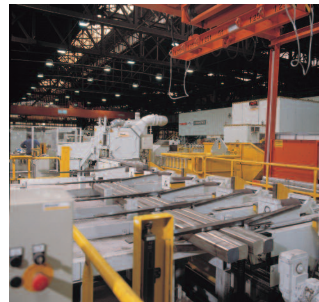
Fig. 33 Chop-stroke abrasive cut-off machine type TS 6 V with integral material handling system at DONETSKIJ METALURGICESKIJ ZAVOD, Donetsk, Ukraine; cutting wheel diameter max. 600 mm (24 in), material: bar, diameter 10 to 25 mm (0-3/8 to 1 in), cutting temperature max. 100 °C (212 °F).
