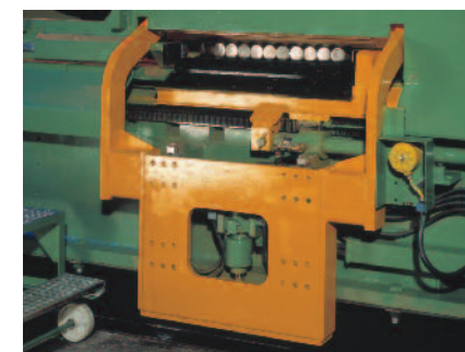
Fig. 23 Material clamping system with hold down bar for layers of bars
