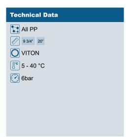
Professional housing completely made in natural PP, with VITON gaskets.
