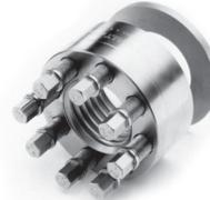
**Superbolt Product:** Confirm jackbolts are lubricated with correct Superbolt lubricant (JL-G, JL-M or JL-AS). New product is lubricated at the factory. Make sure the jackbolt tips are even (or recessed) with the bottom of the nut body.
