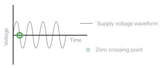
The EPack Controller can accurately detect a zero crossing on the voltage waveform and is able to trigger the thyristor at that moment. This results in less harmonic distortion and RFI, reduction of the dc component, and accurate response to the power demand.
