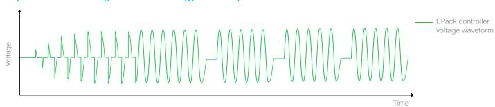
The EPack power controller automatically switches from phase angle to burst firing mode depending upon the ohmic value of the load, for example, during the period of stress when the load is cold. The advanced start-up feature allows smooth start-up with less stress on the load.
