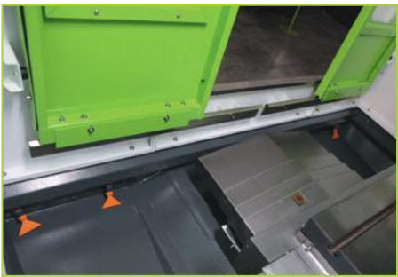
Chip flushing system
