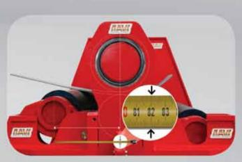
The prebend of the same ULTRA HEAVY plate on much heavier machines have a virtual no flat end at all I despite a more than double side rolls distance (the evidence the flat end ONLY depends on the machine power, and NOT AT ALL on the side rolls distance).
