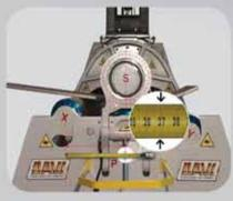
The prebend on a small roll of a ULTRA HEAVY plate (much heavier than the machine capacity) may determine a very long flat end, which cannot be reduced notwithstanding the very short side rolls distance design of the machine.
