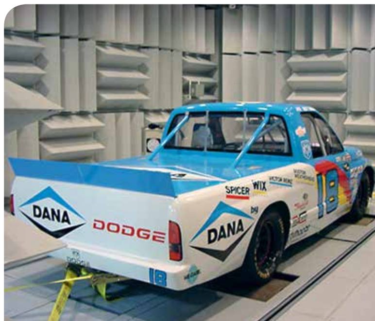
Hemi-anechoic chamber for Dana Trucks, USA
