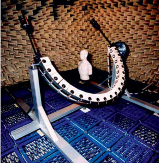
Example of Microdyne® fully anechoic chamber with gridded floor for ISVR in Southampton
