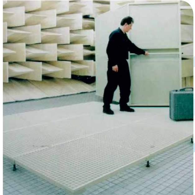
Example of Microdyne® fully anechoic chamber with cable floor plus additional platform for Deutsche Telekom
