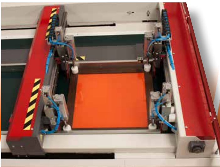
Detail of the pressing step in a model equipped with vertical clamping cylinders acting on the joints of the door (PNEUMATIC LOCK Kit).
