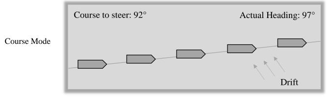
When operating in Course Mode the Autopilot will compensate for any drift by automatically adjusting the actual heading to stay on course.
