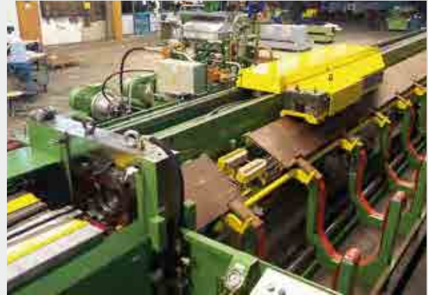
1-fach-Profil- und Stangenziehanlage für Messing- profile mit Push-Pointer Single profile and bar drawing equipment for brass material, equipped with push-pointer
