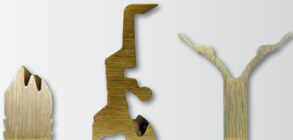
Push-Pull-Pointer für kupferlegierte Profile Push-Pull-Pointer for copper alloyed profiles
