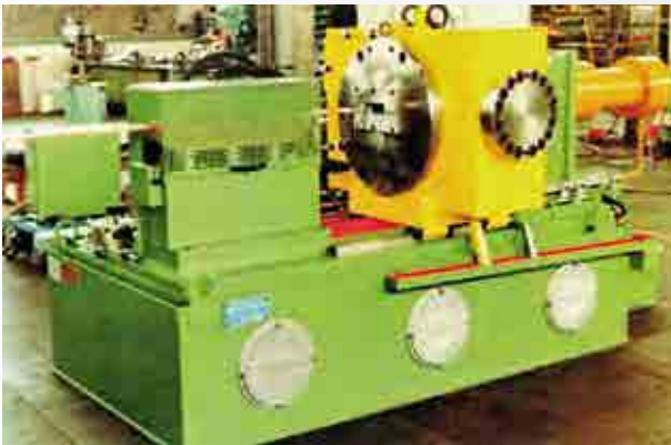
Pull-Pointer für Messingprofile Pull-Pointer for brass profiles
