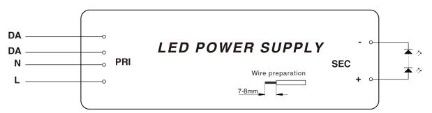
Push DIM wiring diagram
