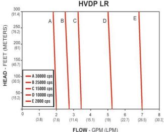
Flow rates are dependent on the properties of the fluid and its ability to flow freely into the pump intake. Expected flow rates for fluids above 30,000 cP are 1 to 3 gpm (3.8 to 11 lpm).
