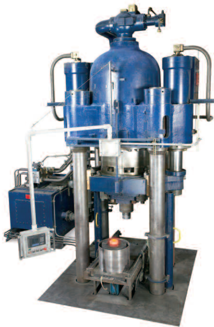
A 2,500 Ton Press Is Used To Rapidly Consolidate Dynaforge Monolithic and Bi-Metallic Shaped Components
