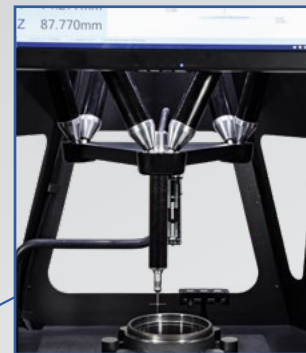
Robust design utilising linear motors and mechanical bearings.
