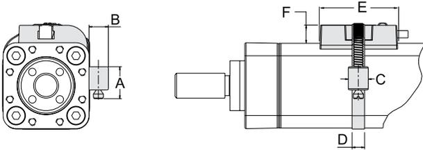
The bracket can be installed over the left or right corner of the cover tube surface under which the sensor magnet travels. The bracket comes with all necessary items to mount it to the actuator. Sensors are supplied separately, see list for available suitable sensors.
