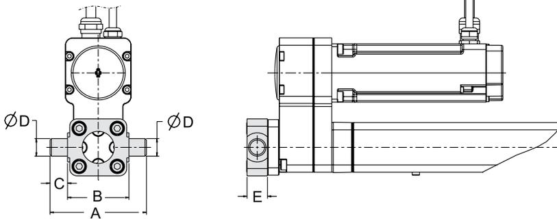
The fixed front and rear trunnions consist of a plate with two shafts and come mounted from the factory if the ordering code states that the unit shall be equipped with one. They can also be ordered as a separate parts (all necessary actuator attachment screws are included) using the part numbers. The rear trunnion can only be mounted on to the belt gear on parallel style actuators.
