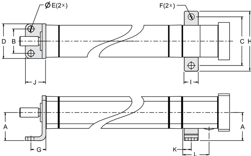
The foot mount consists of a front and rear bracket and comes mounted from the factory if the ordering code states that the unit shall be equipped with one. It can also be ordered as a separate part (all necessary actuator attachment screws are included) using the part number.
