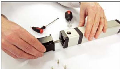
Insert motor shaft into coupling
