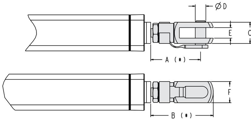
The front clevis comes mounted from the factory if the ordering code states that the unit shall be equipped with one, but it can also be ordered as a separate part using the part number. To be able to mount a separate front clevis the extension tube must be equipped with a male threaded rod end.
