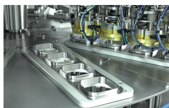
Strong and light cassettes in aluminium and stainless steel.
