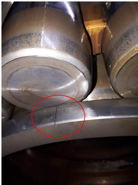
Image 3. Cracked inner race.
