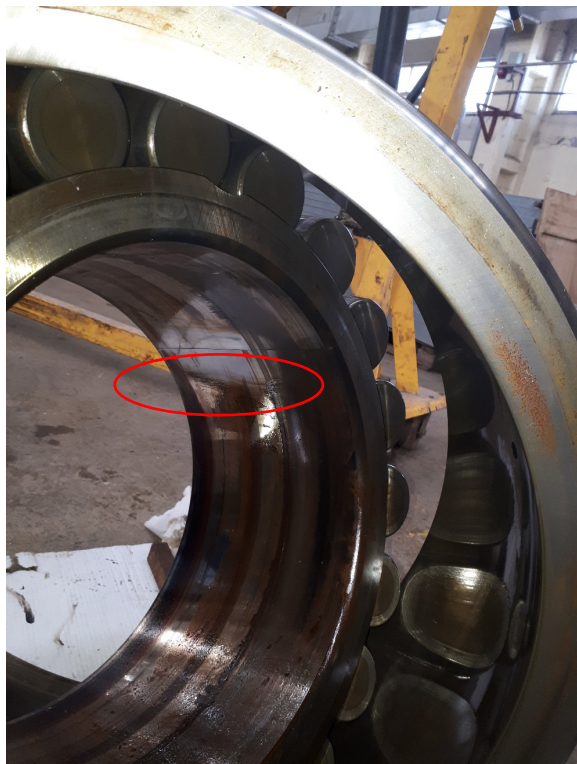
Image 2. Cracked inner race.
