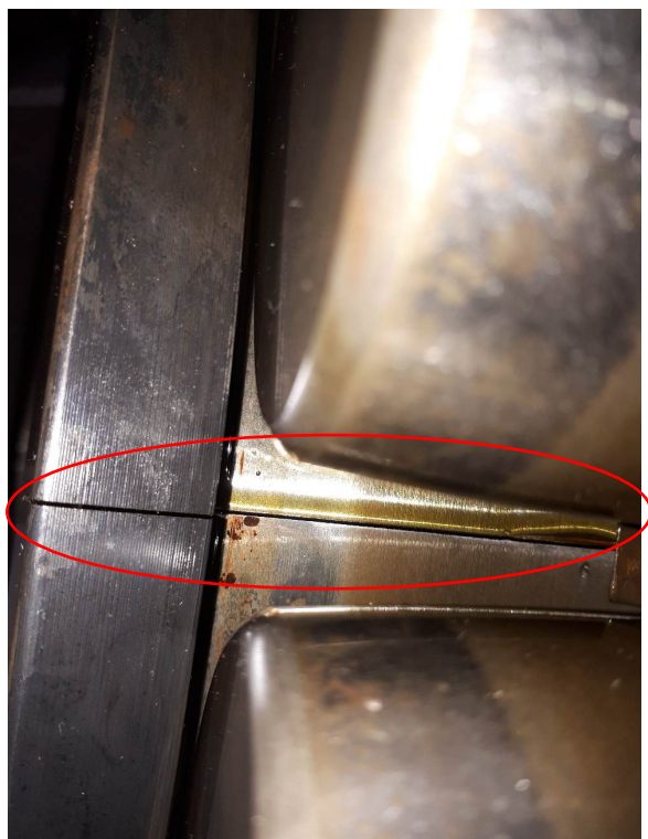
Image 4. Cracked inner race.
