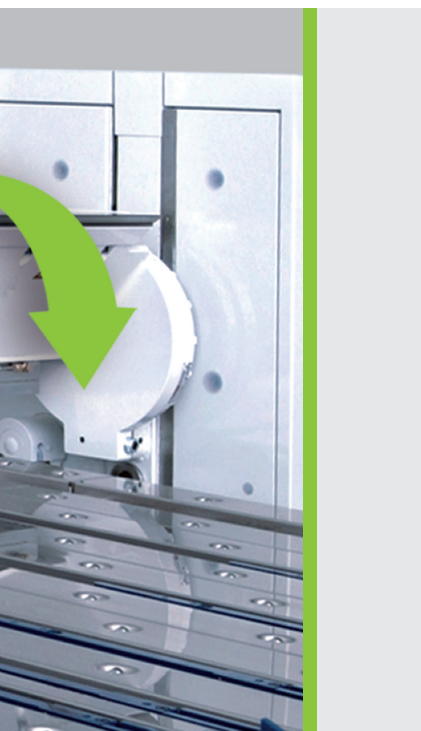
With a rotating clamping beam the MPB keeps a second set of tools in readiness.
