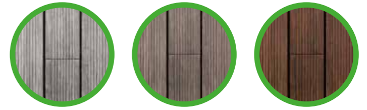
after 12-18 months weathering after brushing & cleaning after treatment with decking oil
