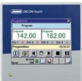
elements and acquiring their surface temperature. Based on the surface temperature, the maximum heating output for the power controller is defined. The external control loop controls the furnace temperature. The two-channel process and program controller JUMO DICON touch meets all the designated requirements here. All important process parameters can be displayed on a process screen. Communication with a higher-level PLC via fieldbus is also possible.
