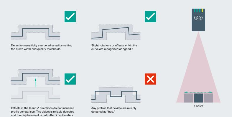
Reliable detection of object contour, positioning, and distance
