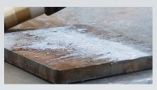
After the attachment is removed, operators can reduce the amperage on the system and wash any remaining material away without digging into the workpiece. FlushCut washing further reduces the need for grinding.
