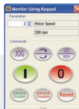
Monitoring and command window using virtual keypad. Start/Stop function, JOG, local / remote, Reverse and reset
