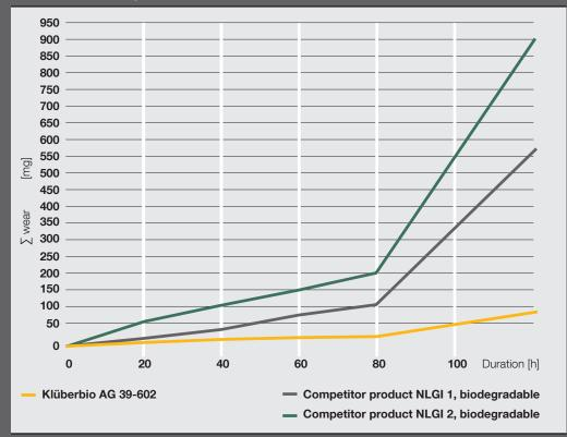
Klüberbio AG 39-602 shows lower wear rates than other open gear lubricants.
