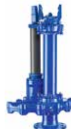
Series 29/78 Underground fire hydrant Free flow Single shut-off DN 80 PN 16 750-1500 mm Ductile iron
