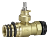
Series 343/81 Ball valve with Supa Lock™ spigot end/BSP thread 1"-1 1/2" DN 32, PN 16 Brass
