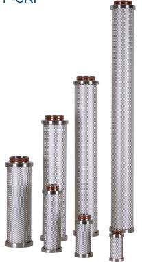
The P-SRF is a wounded depth filter with inner and outer guard end caps made of stainless steel. Consisting of a three-dimensional borosilicate depth media, the P-SRF achieves a void volume of 95%, ensuring a high containment capacity at high flow rates and low differential pressure. A retention rate of >99.99998% related to 0.2  $\mu$ m is achieved during operation.
