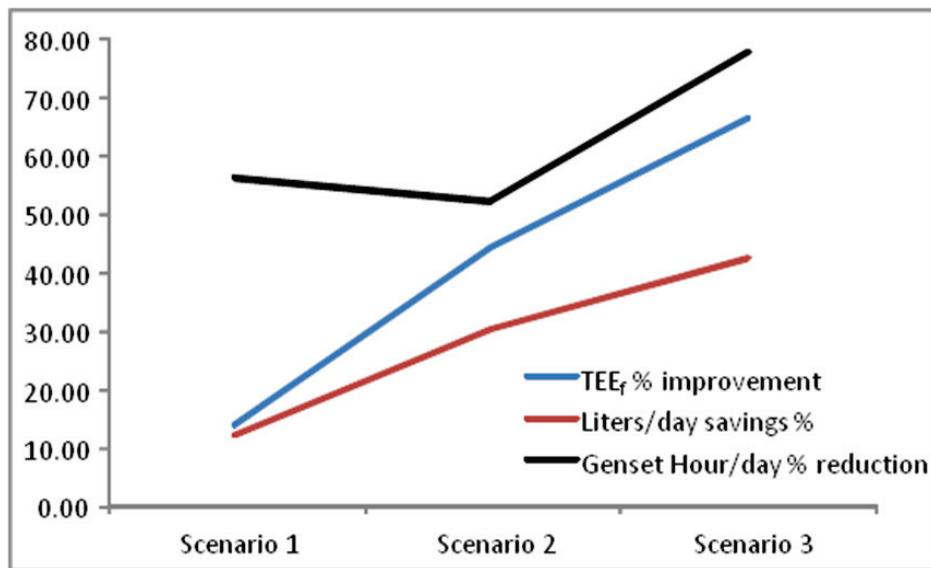
The Cummins hybrid power system aims to maximize overall system efficiency by improving the ratio of available energy utilized by transmission loads to the fuel consumed in KWh. Additionally, it provides features such as battery condition monitoring and maintenance predictability that improve the overall lifecycle performance of the system.
