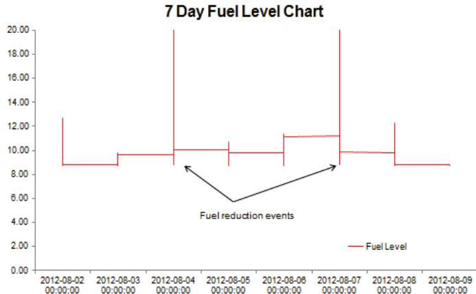
Conventional approach to hybrid power systems focuses on reducing generator set run time (in hours) and/or monitoring fuel pilferage as the primary means to OpEx reduction.
