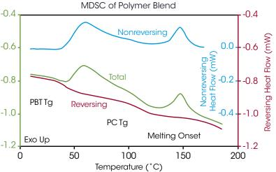
Deconvolution of an Overlapping Glass Transition and
