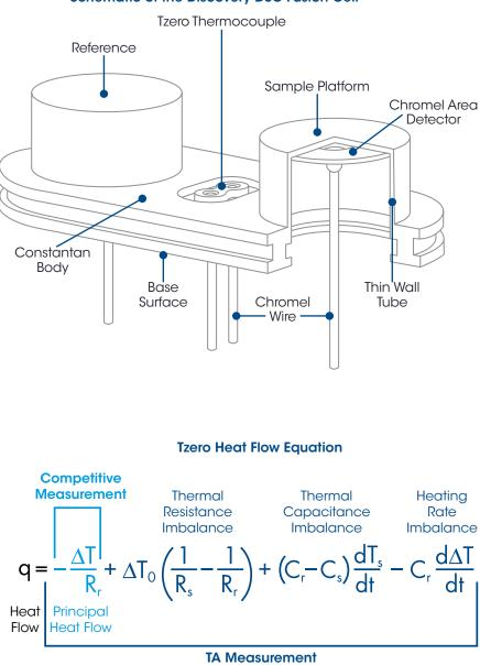
Schematic of the Discovery DSC Fusion Cell™
