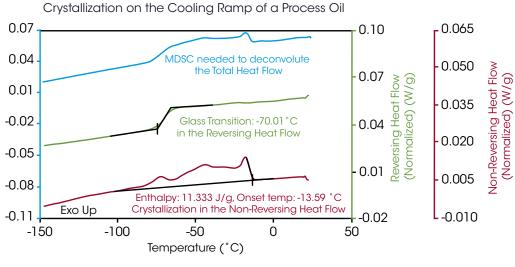
This process oil exhibits a variety of overlapping transitions, making interpretation of the Total Heat Flow complicated. On the cooling ramp from 25 to -150 °C, MDSC effectively separates crystallization into the Non-Reversing Heat Flow and the glass transition into the Reversing Heat Flow. Gain confidence in data interpretation with the help of MDSC!
