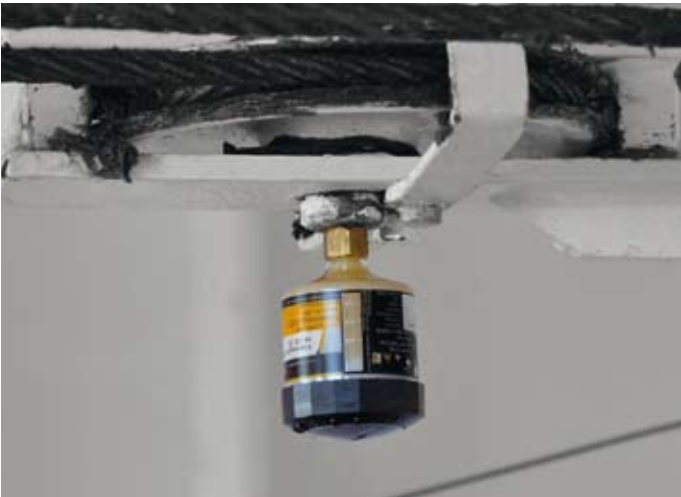
Life raft davit applications: – rolling bearings – cable pulley Lubrication system: Klübermatic FLEX 60 cm³
