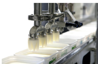
Cup filling station with drip free nozzles
