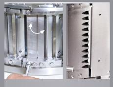
Adjustable gate flexes as top/ bottom adjustable screws are turned to provide microadjustability of slice thickness
