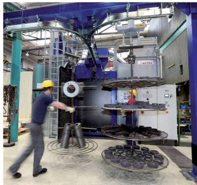
In drum shot blast machines small work pieces are blasted as bulk goods. Thus they can be used in production lines or for stand-alone configurations.
