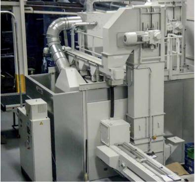
Travelling grate shot blast machines are designed for gentle transport of all kinds of work pieces. In this case we show springs being shot peened.
