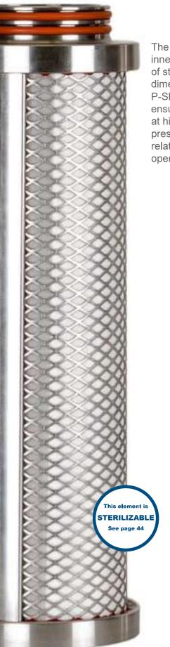
The P-SRF is a wounded depth filter with inner and outer guard end caps made of stainless steel. Consisting of a three-dimensional borosilicate depth media, the P-SRF achieves a void volume of 95%, ensuring a high containment capacity at high flow rates and low differential pressure. A retention rate of >99.99998% related to 0.2  $\mu$ m is achieved during operation.
