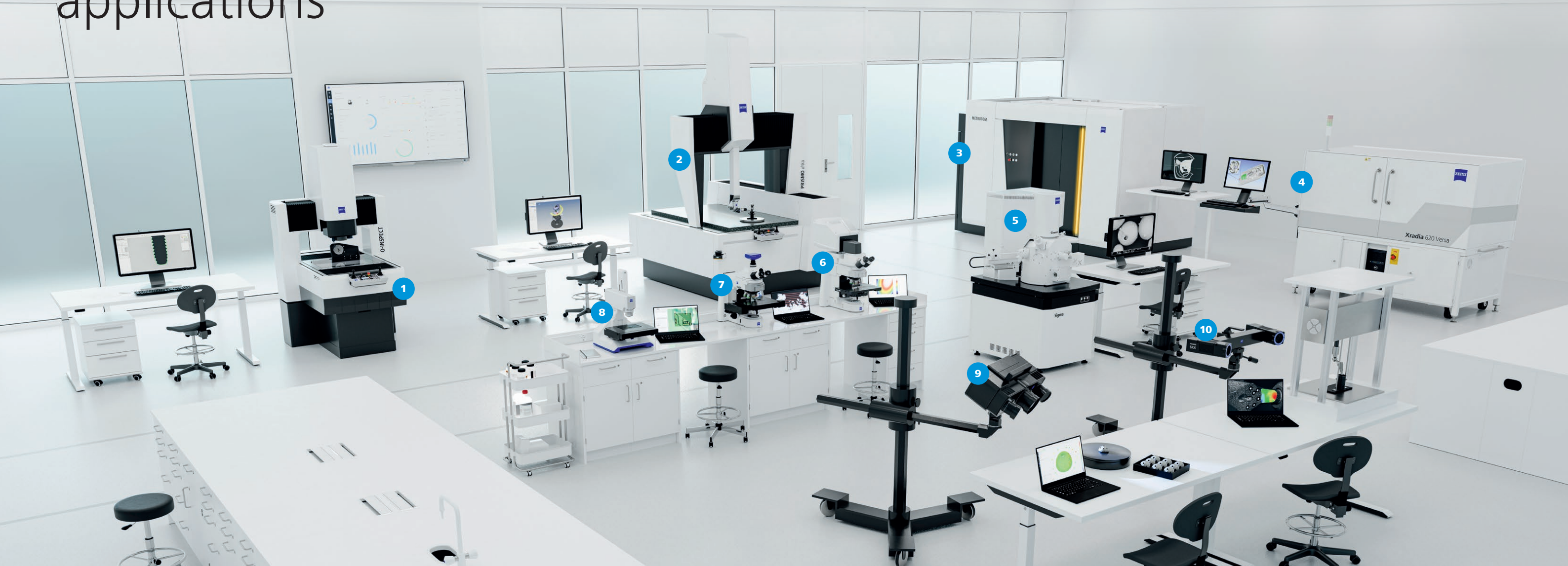
1 ZEISS O-INSPECT 2 ZEISS PRISMO 3 ZEISS METROTOM 4 ZEISS Versa 5 ZEISS Sigma 6 ZEISS LSM 900 7 ZEISS Axio Imager 8 ZEISS Smartzoom 5 9 ZEISS ATOS 5 10 ZEISS ARAMIS
