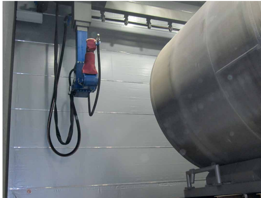
Blast booth with "ReCo-Blaster"® for cleaning components of wind energy plants
