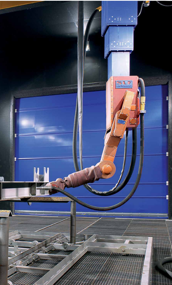
Blast booth with "ReCo-Blaster"® for cleaning components of wind energy plants
