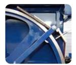
The cooper cleaners are installed in a way that the sawdust will inmediately get out of the sawhead and will not get onto the sawblade itself.
