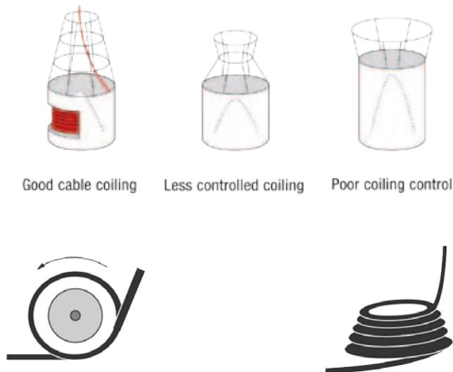
The cable has to be laid, from the bottom of the basket, in anticlockwise direction starting from the outer layer of the original cable drum.
