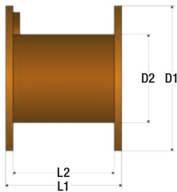
On the above table you can find our most common types of drum. For each one also we provide internal and external dimensions, weight, bulk space and volume. Please consider that a staved drum increase its dimension D1 of 50 mm in total.
