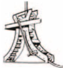
As a general note, you have to absolutely avoid any abrupt changes of the bending radius (often this is due to a not enough long angle of deflection of the roller guide arc). These changes lead to a punctual overpressure that results into a cable breakage.
