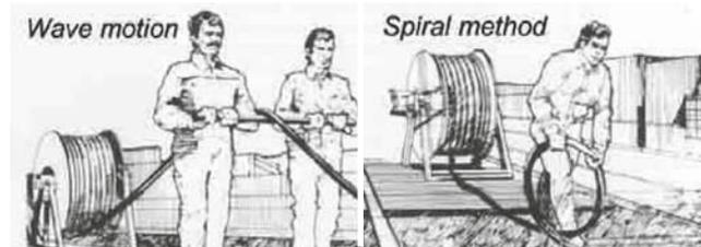
The spiral will be rolled to the free end of the cable in order to remove any twisting. This action must be performed again for each founded twisting. Then re-anchor the cable to start operation. If during the first test-running of the equipment you still find a slight or residual twisting, lead the machine to the end run then un-anchor the cable (eventually cutting 25/50cm of cable) and eliminate the torsion. After this, re-anchor the cable and have a final check.
